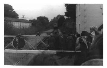
Finally, the diesel-electric multiple-unit 3car set arrives from the Uddens & Wimborne direction. These trains were part of the British Railways Class 205 fleet – the primary motive power being a diesel engine generating electric power which was then used to drive the wheels. They were long in service, first units appearing in 1957, finally bowing-out in 2004. Several of these trains are now in private hands – being put to use on 'heritage' railways.
